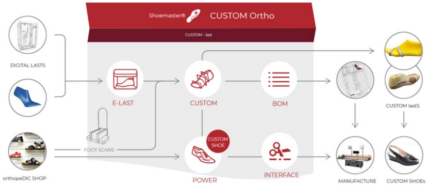
Figure 26. Shoemaster custom technological process for the production of orthopedic shoes (source: www.technorg.hu )
