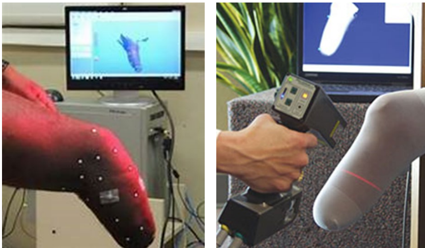
Figure 10. Scanning a mutilated limb to make a prosthesis (source: 3dprint.com)
