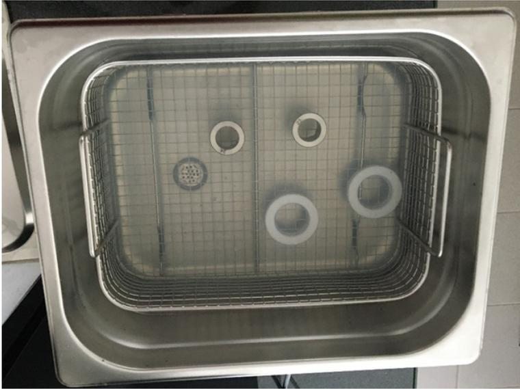
Figure 2. Cleaning shafts and seals in an ultrasonic bath.
