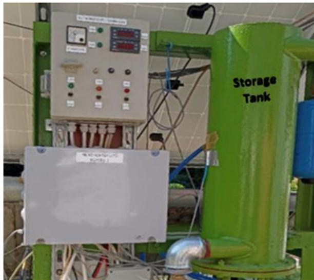
Figure 3. Arduino-based control unit and the storage tank
