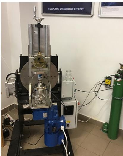
*Figure 5. 3-body abrasive wear testing by sand-pot test rig.*
