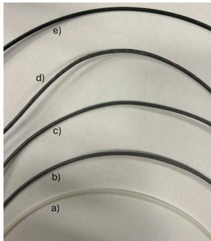
Figure 2. Pure PLA and graphite-enriched PLA fibers (a, 0% graphite + PLA, b, 0.5% graphite + PLA, c, 1% graphite + PLA, d, 2% graphite + PLA, e, 5% graphite + PLA)
