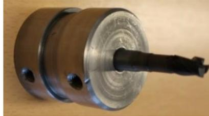
Figure 6. The tool holder insert with the fixing holes is made for a tool diameter of 6 mm
