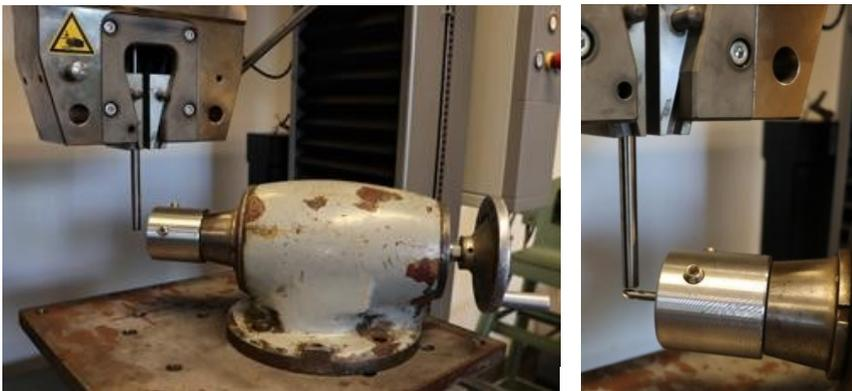
Figure 9. Planned Measurement assembly and load zone
