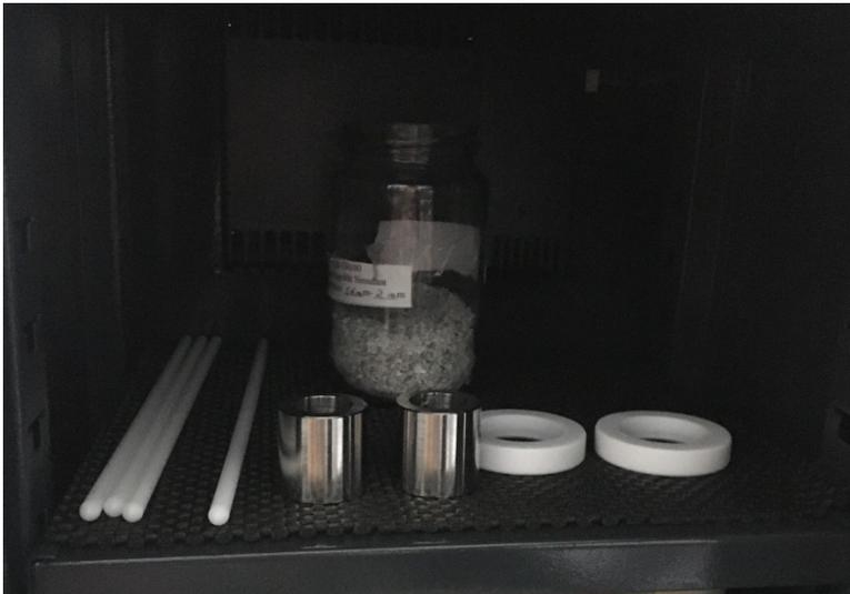
Figure 3. Drying shafts, seals and Lunar regolith in the drying chamber.
