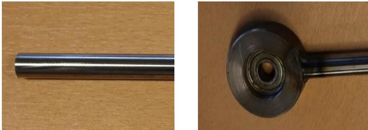
Figure 7. Push rod with cylindrical solid and bearing roller end
