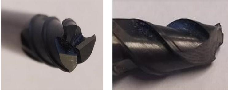
Figure 12. Photos of the tool used for validation measurement (Frais P5230 Ø6) before (left) and after (right) the breakage test
