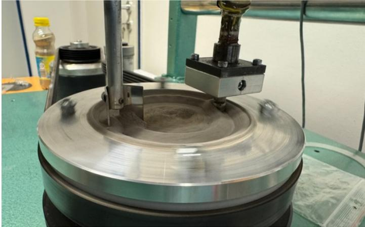
Figure 3. The abrasive pin-on-disc method during measurement
