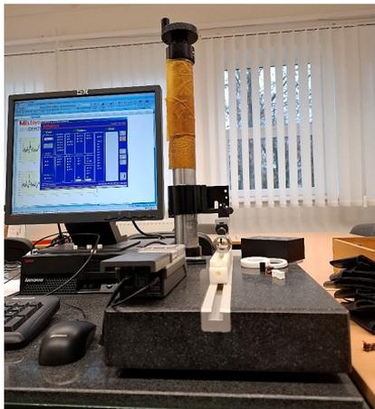
*Figure 4. Surface roughness test of stainless steel shaft sample*
