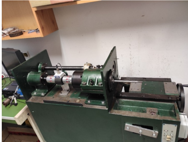
Figure 2. new shaft in the old bearing housing
