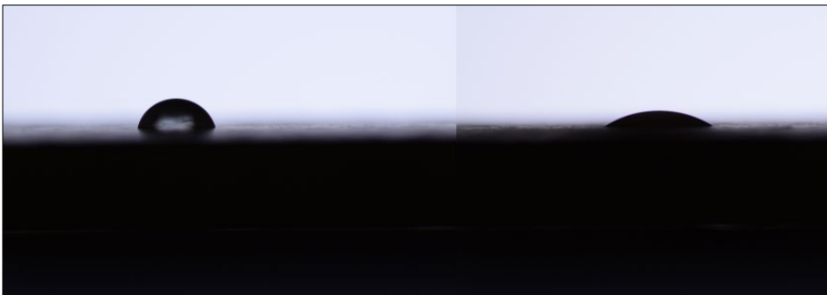
Figure 3. The result of the plasma preliminary experiment: the untreated surface on the left, the treated surface on the right.
