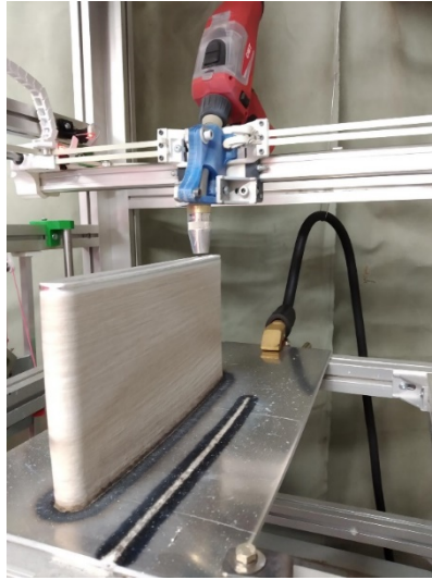
Figure 2. 3D metal printer developed by the research group of the Faculty of Engineering and Computer Science at the University of Pécs. (Gyula Ferenc Vasvári, 2021)
