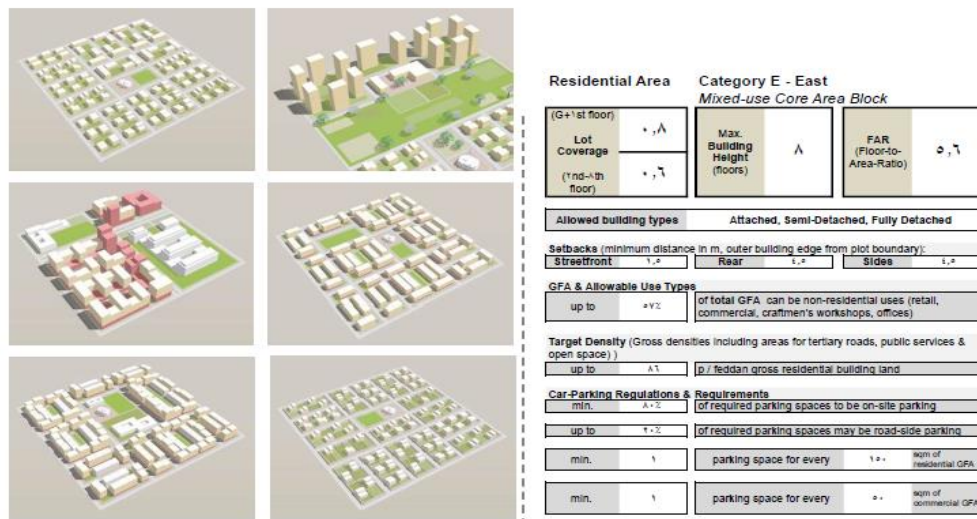
Figure 25 :Building conditions and land use in Al Montazah district as example for the land use and building conditions in Alexandria master plan 2032, Source: (General organization for physical planning, 2020).
