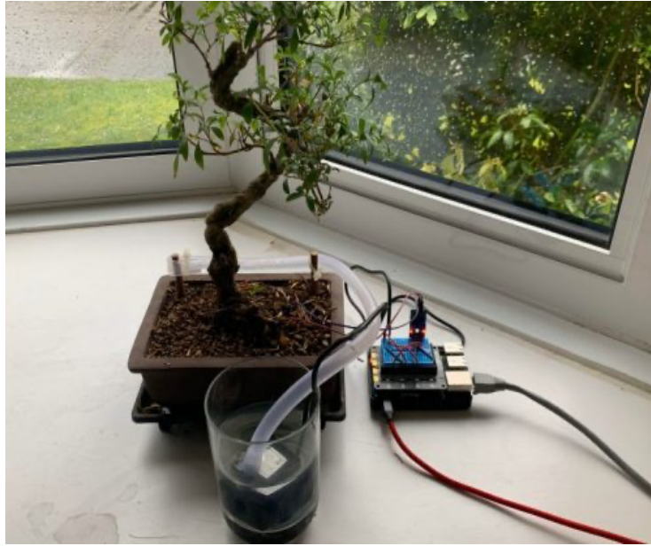
Fig. 2.7. Soil moisture levels measured by a capacitive soil moisture sensor (Harry-Lees, 2020).
