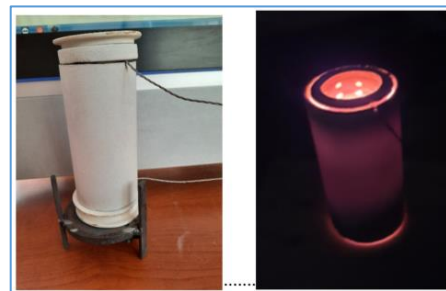
Figure 6. Directly electrically heated, air-inlet laboratory reactor, maximum operating temperature: 1300 °C (MATE lab)
