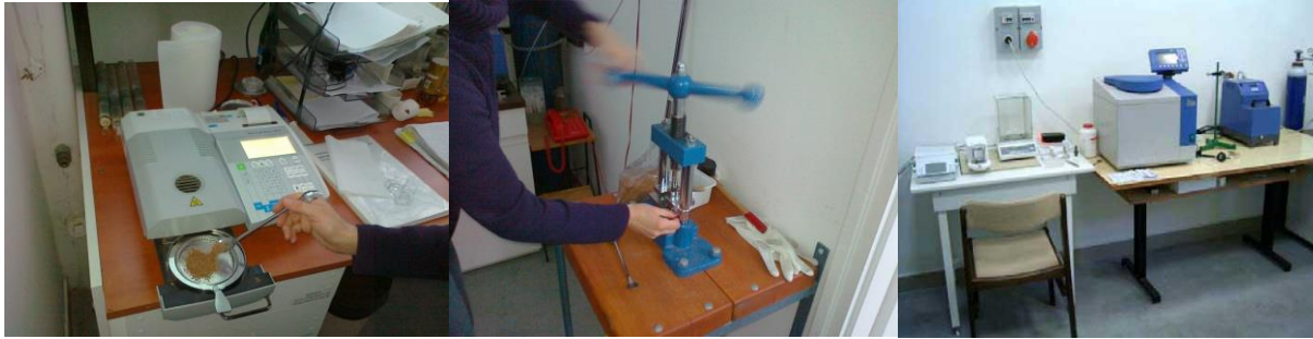
Figure 1. METTLER TOLEDO moisture gauge, compression press, IKA-WERKE C2000 calorimeter (MGI lab)
