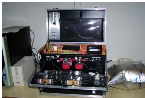
Figure 3. VISIT 03H gas analyzer (MGI lab)
