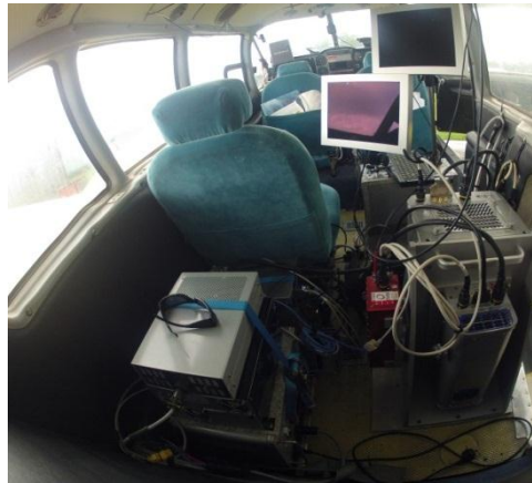
Figure 2. AISA Dual hyperspectral sensor set up in Piper Aztec aircraft
