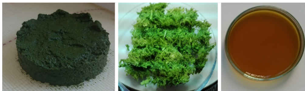
Figure 1: Alfalfa green biomass originated fractions: leaf protein concentrate (LPC), green fibre, brown juice
