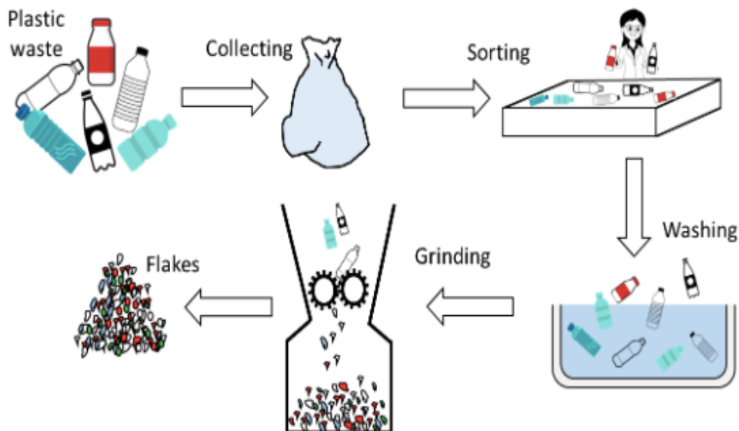
Figure 5 - scheme of the basic principal steps in a mechanical recycling process
