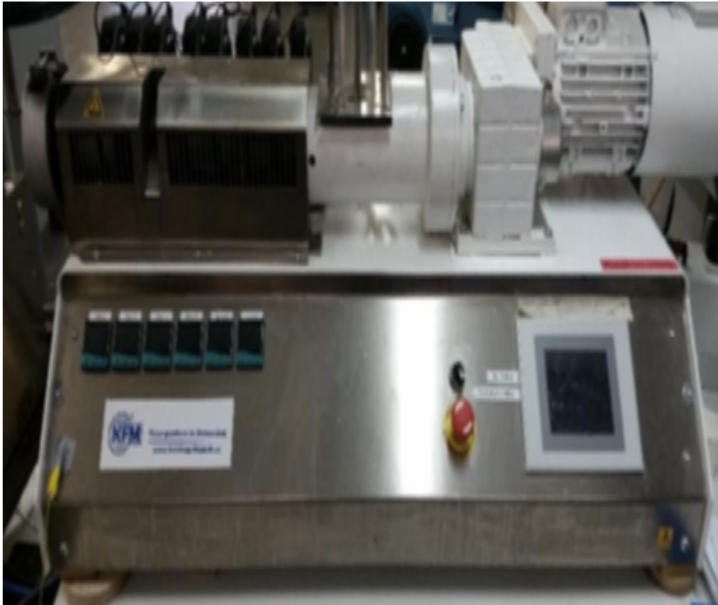
Figure 18 - sample of extrusion machine during the preparation of specimens
