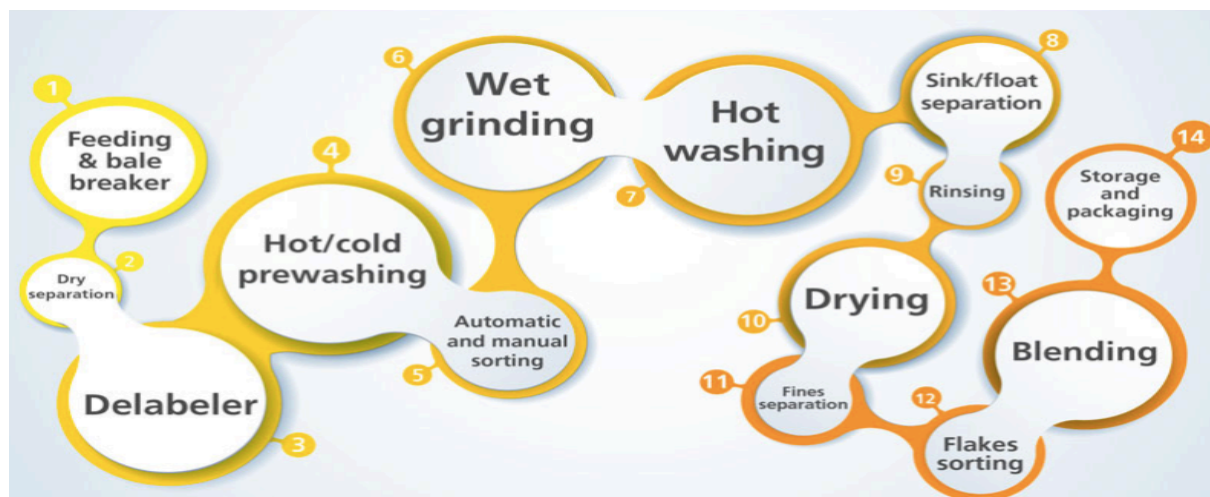
Figure 14 - PET plastic recycling steps
