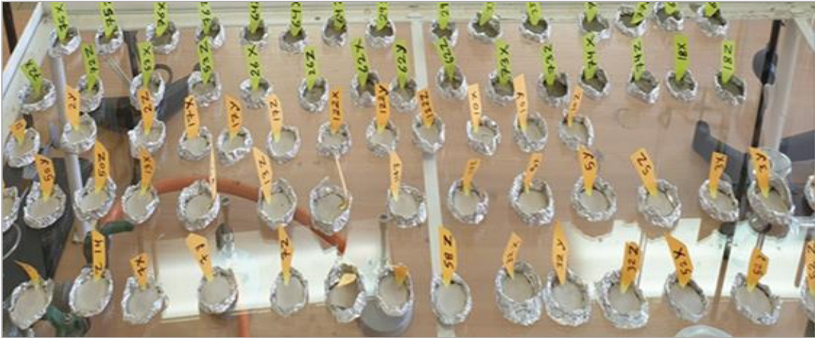
Figure 12. Mortar-incorporated adsorbed ash composites
