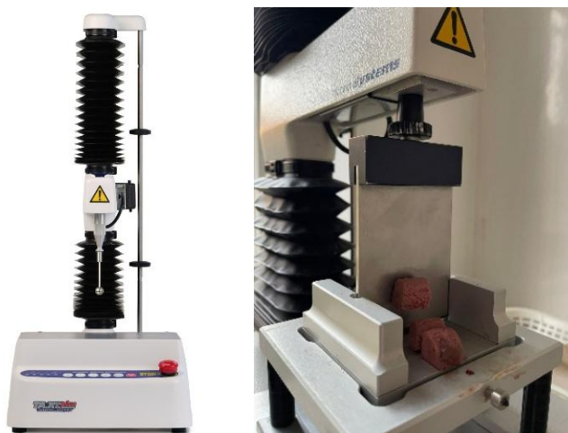
Figure 10. TA.XT Plus Texture Analyzer (Stable Micro Systems) used for the measurement and the measurement process during the texture analysis of wild red deer samples (Photo by the author)
