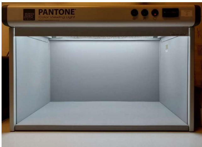
Figure 7. Just Normlicht Pantone Color Viewing Light BASIC 3 light booth (own photo)
