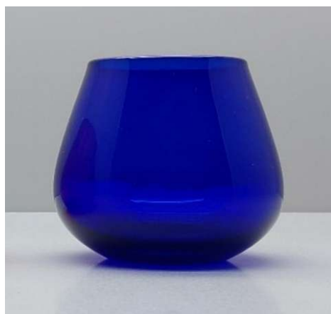
Figure 10. Standard cobalt blue olive oil testing cup (ISO 16657:2023) (own photo)
