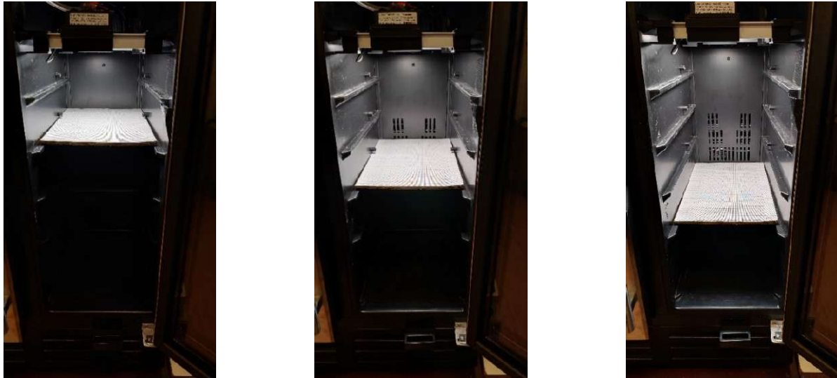
Figure 1. Measurement grid points applied to horizontal surfaces on the upper, middle, and lower levels of the right chamber of the climate chamber illuminated by the Ledium Black Sparkle Modular64 Base (own photo)
