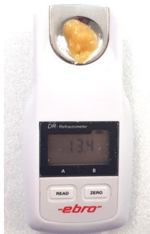
Fig. 3.6. DR-10 type digital refractometer
