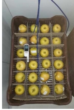
Fig. 2. The Ebro EBI 300 TH Multi-Use USB Data Logger for temperature and humidity measurement
