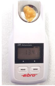
Fig. 5. DR-10 type digital refractometer
