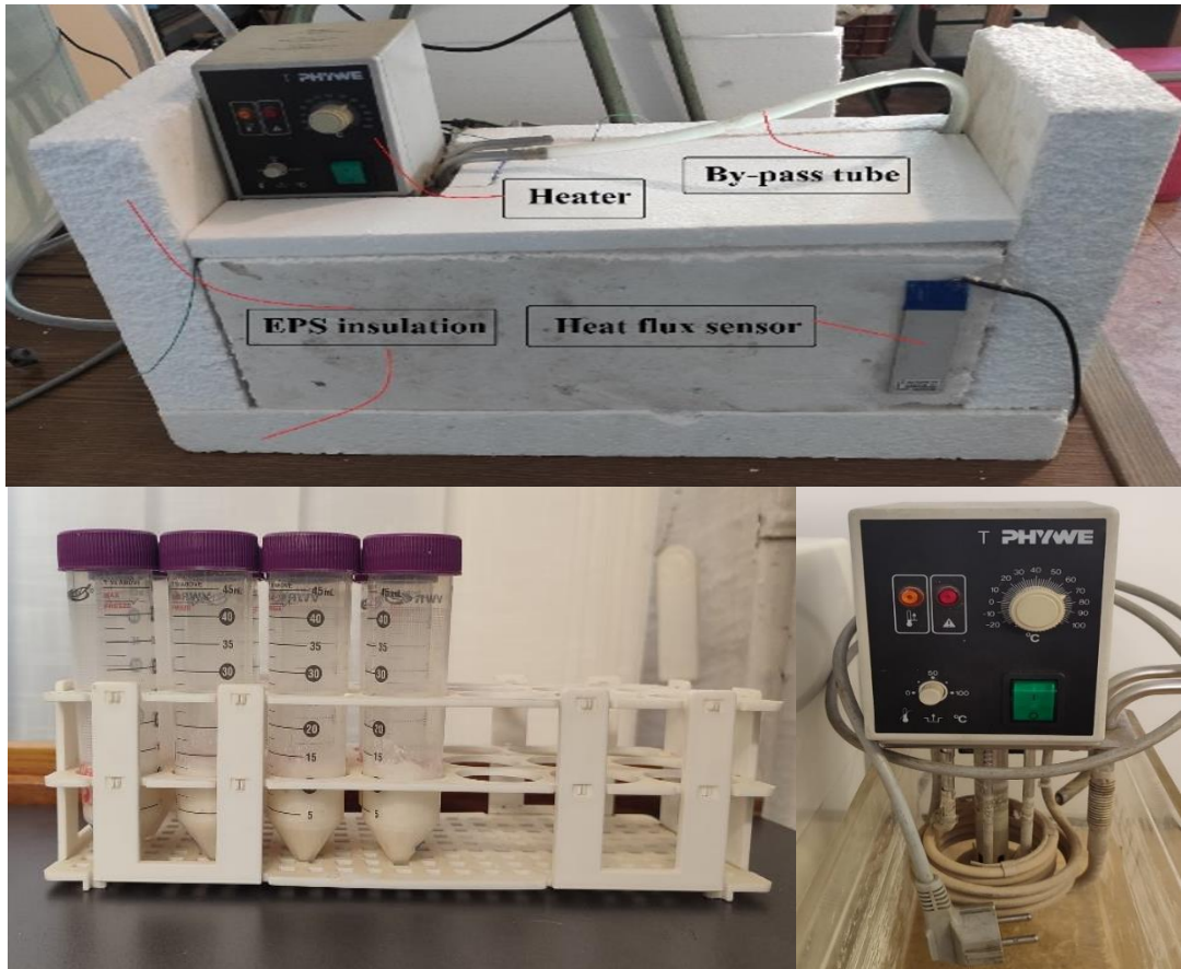
Fig. 3.1. The insulated thermal tank with PCM tray and heater
