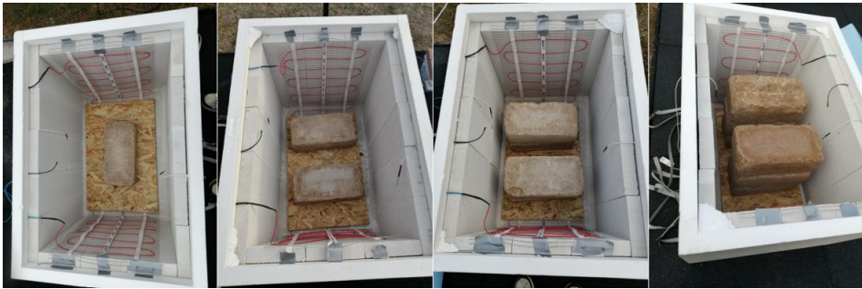
2.3. Fig. Modification of heat storage masses before different measurements
