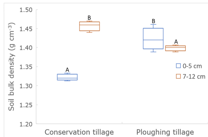
Figure 13. Soil bulk density ( g\ cm^{-3} ) in the CT and PT at 0-12 cm depth for the growth stages V3 in the growing season of 2022, n=4 .
