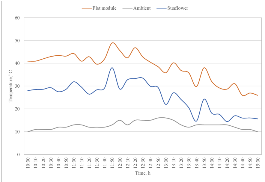
Fig. 15. PV systems temperature measurement ( \alpha=45^\circ )
