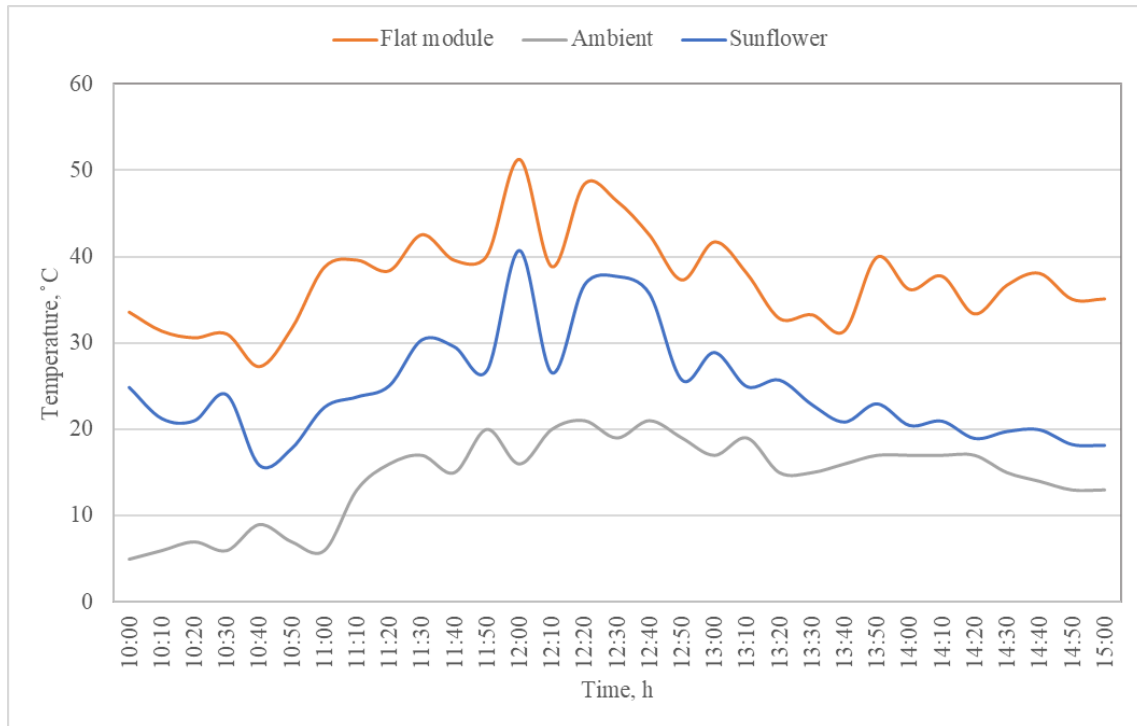
Fig. 4.13. PV systems temperature measurement ( \alpha=30^\circ )
