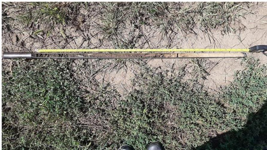
**Figure 3.5. Pürckhauer type soil core sampler in Józsefmajor (cropland) (26/08/2020)**
