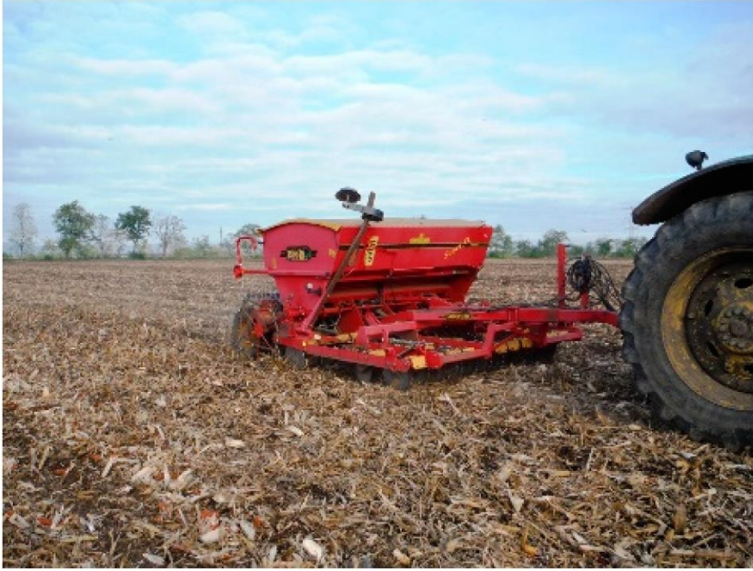
Figure 3. No-till planter at the JM experimental farm near Hatvan (Source: Dekemati Igor)
