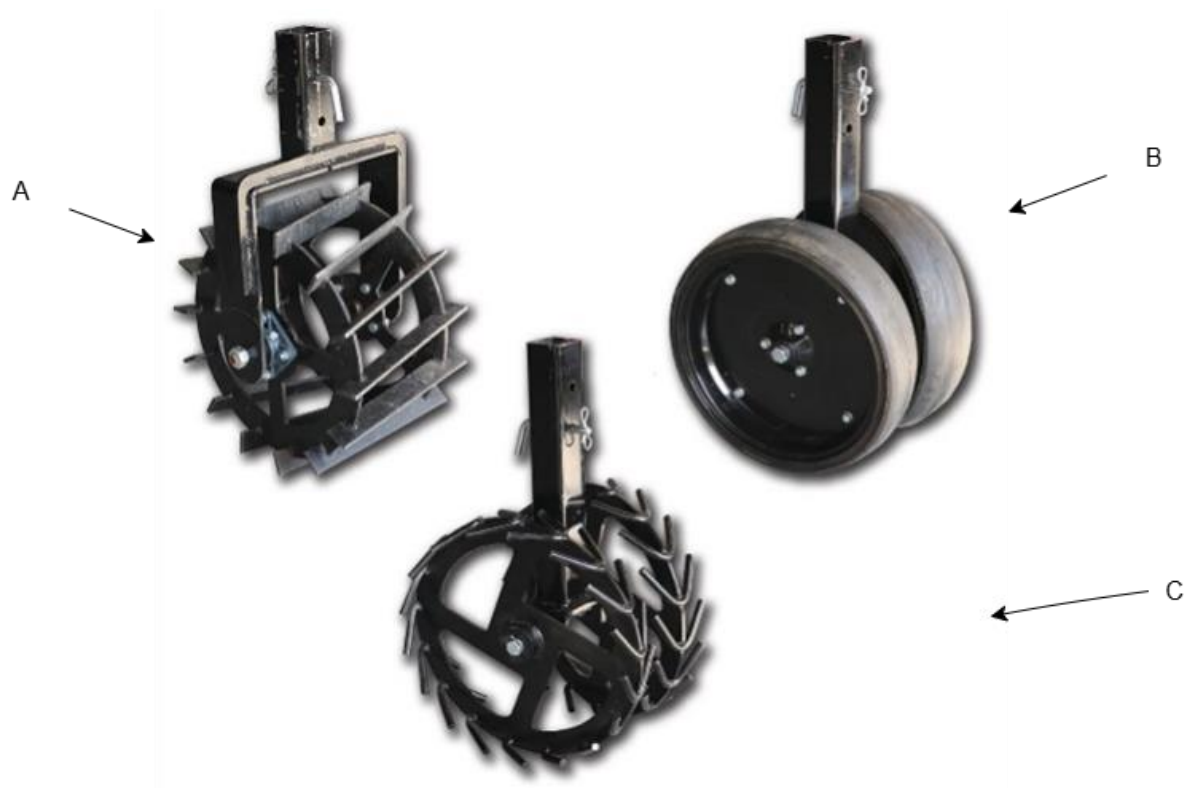
Figure 1. Different strip soil tillage roller crumblers. A-Cleated roller, B-Rubber press wheel, C-The steel wheel. Source: (http2, 2025)
