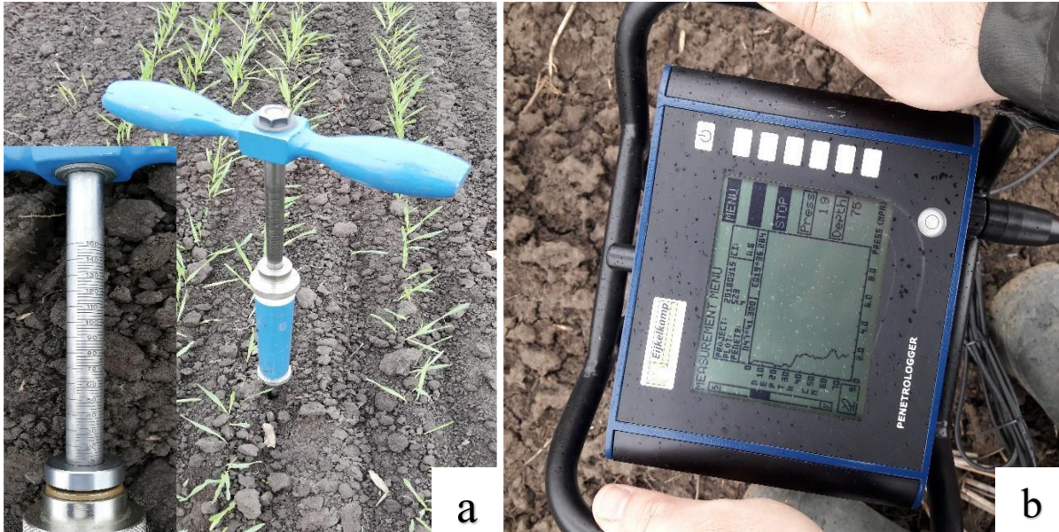
Figure 10. Szarvas-handheld type (a) and Eijkelkamp (b) penetrometers . Photos by Igor Dekemati
