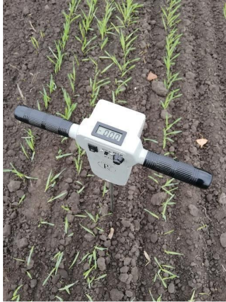
Figure 9. Soil moisture meter, a PT-I type gauge (Kapacitiv Kft, Budapest, Hungary) . Source: Dekemati (2020)
