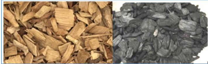
8. Figure Hardwood chips before and after carbonization
