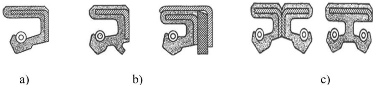
Fig.2.11. Shows several sealing: a) single seal, b) auxiliary sealing lip ,and c) double seal (Neale, 1995).
