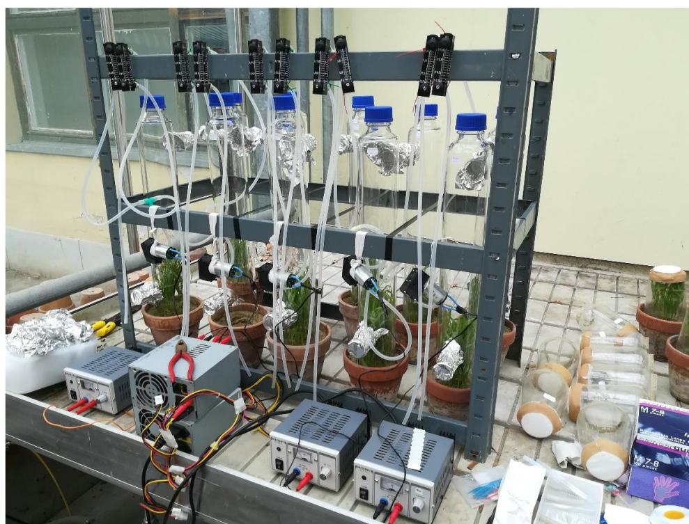
Figure 10. Sampling setup for DHS sampling consisting of eight pots of wheat plants and two blank pots under glass cups with air in- and outlets located in the bottom and the top
