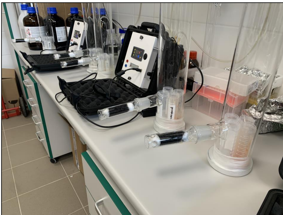
Figure 9. Picture of the open-loop-pull-type DHS sampling system during the competitive binding site investigation, as described in Section 4.2.4
