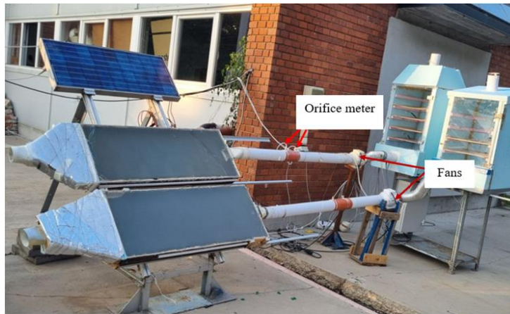
Fig. 2. The setup of the drying system
