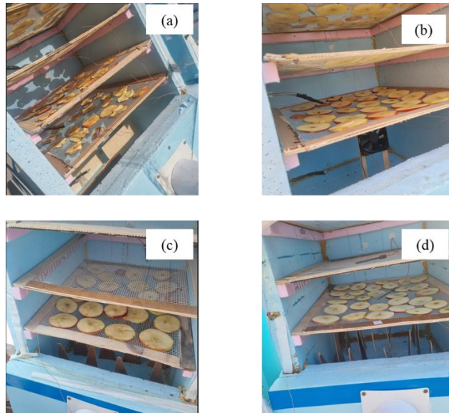
Fig. 3. Flow enhancement materials integrated within the drying chamber: rectangular baffles (a), swirler (b) and triangular baffles (c, d)
