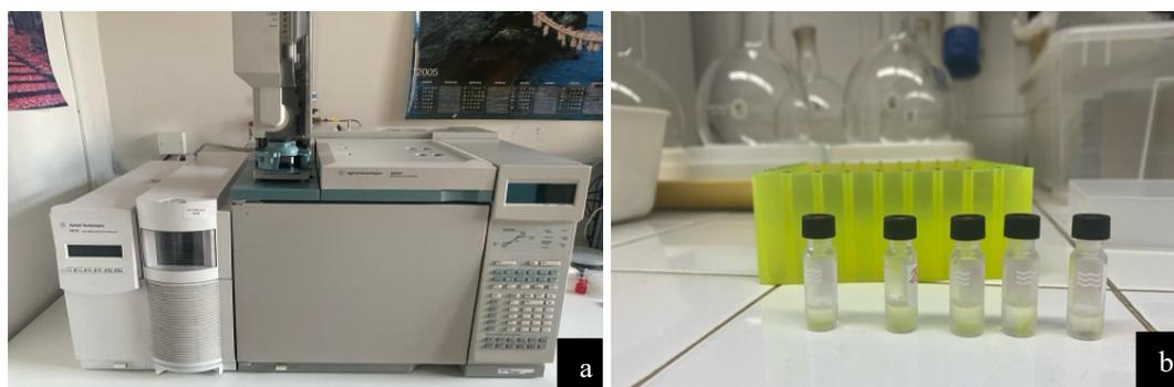
**Figure 13** Agilent Technologies GC instrument (a) for EO chemical analysis (b) (Photo: Kandoudi, 2022)
