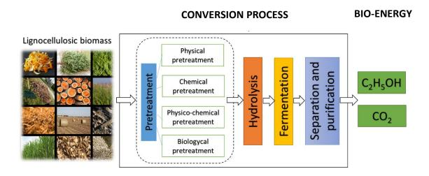
Figure 2.7 Ethanol conversion process from lignocellulosic biomass
