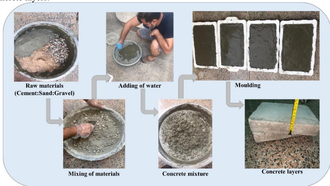
Fig. 3.5. Fabrication procedure of concrete layers
