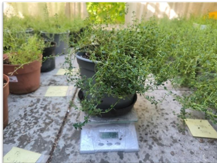
Figure 3. Measuring plant weight to determine water requirements for SWC per irrigation (Budapest, 2025).
