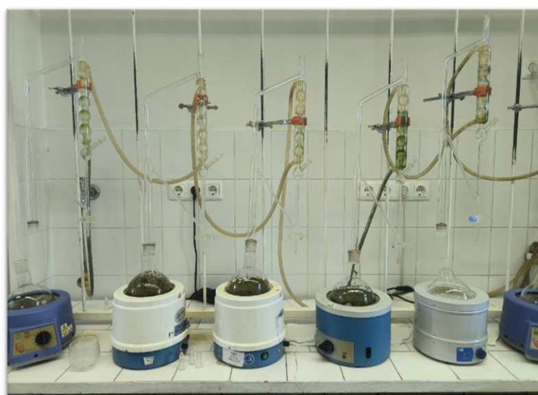
Figure 7. Clevenger-type apparatus used for the hydrodistillation.
