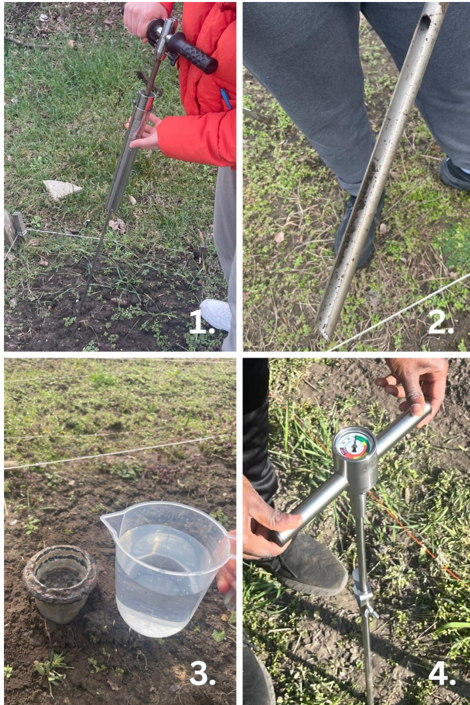
Figure 10: Soil Penetrometer (calibrated in kPa) 1., Soil Auger for Moisture Sampling 2., Infiltration Ring 3., and Soil Penetrometer (color-coded scale) 4.
