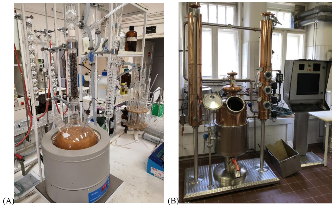
Figure 8. (A) Glass distillation system and (B) steam-heated still equipped with a rectifying column and dephlegmator
