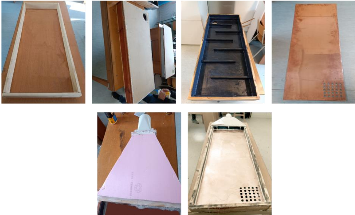
Fig. 3.6. Fabrication process of DPSAC
