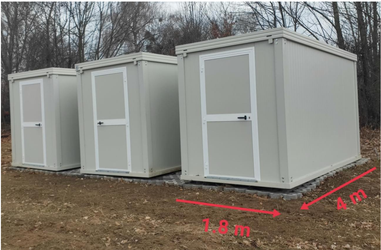
Figure 13. The controlled growth chamber at the experimental field
