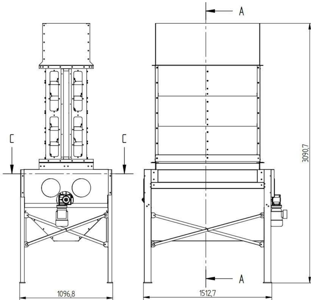
Figure 2.2.: The structure and main dimensions of the model dryer
