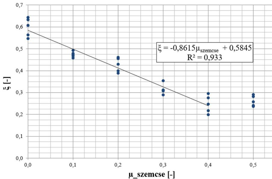
Figure 3.2.: Material flow unevenness as a function of the grain-grain friction coefficient for a  $27^\circ$  lamella inclination angle
