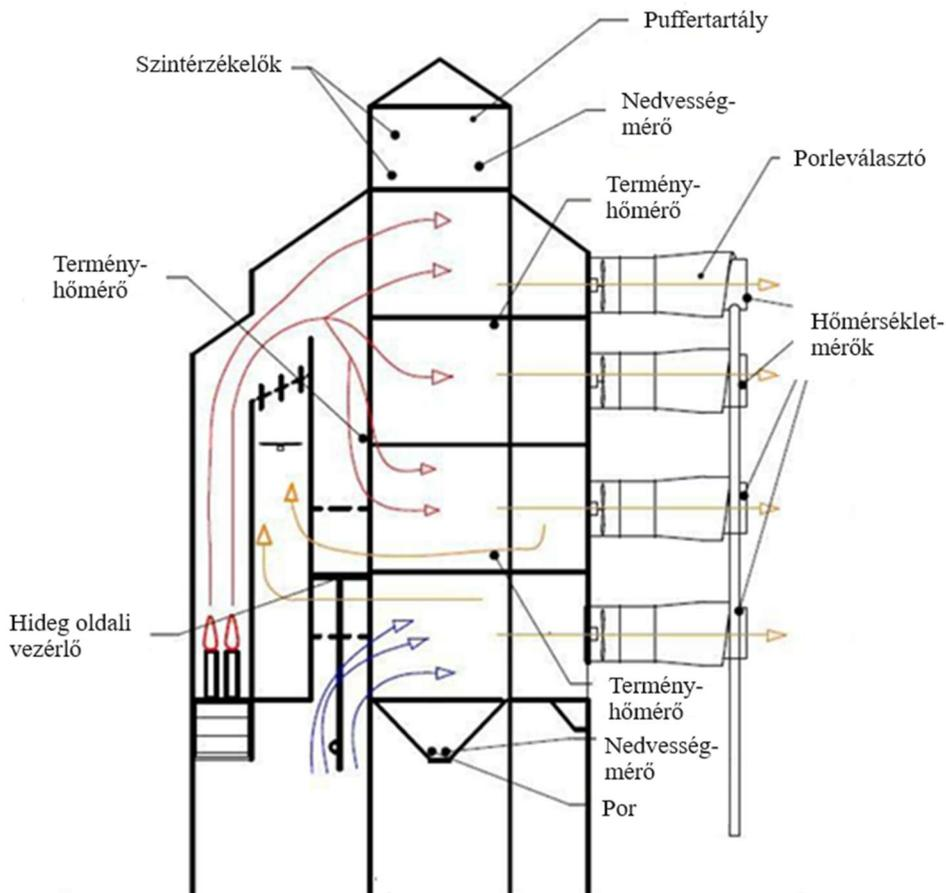
Figure 2.1.: Main components of the industrial dryer
