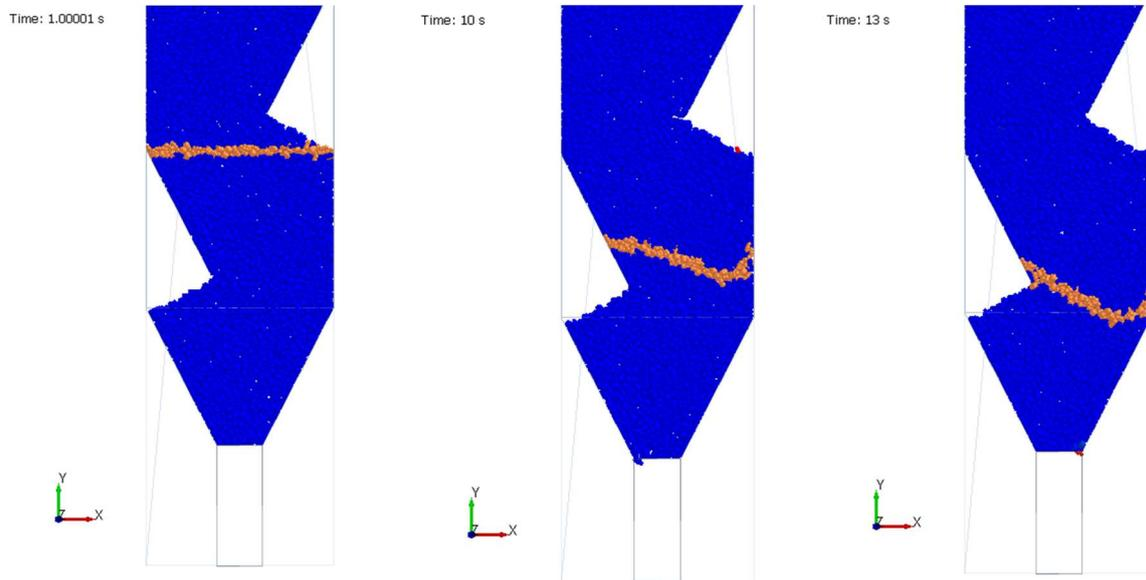
Figure 2.6.: The position of the marked bands at the initial time (1 s), and after 10 s and 13 s for a 27° lamella inclination angle
