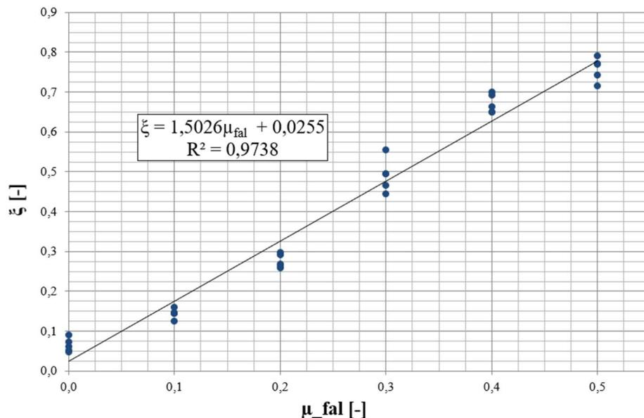
Figure 3.1.: Material flow unevenness as a function of the grain-wall friction coefficient for a  $27^\circ$  lamella inclination angle
