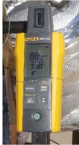
Fig. 3.17 Fluke FLK-IRR1-SOL solar irradiance meter
