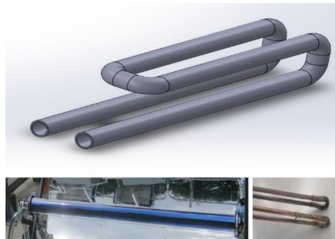
Fig. 3.9. Loop evacuated absorber tube
