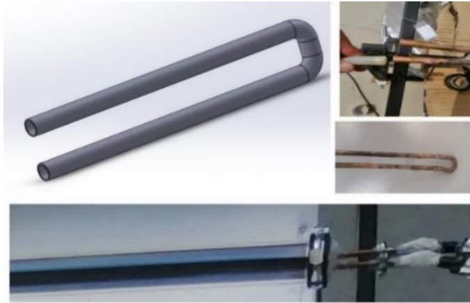
Fig. 3.8. Double evacuated absorber tube
