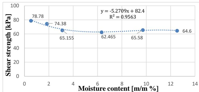
**Fig. 3.5.** Shear strength of the tested sand soil as function of moisture content (70 kg/223.68 kPa initially applied load/stress, and 30 kg/95.86 kPa is used with shearing); shear strength at 1.84 % is included in the figure.
