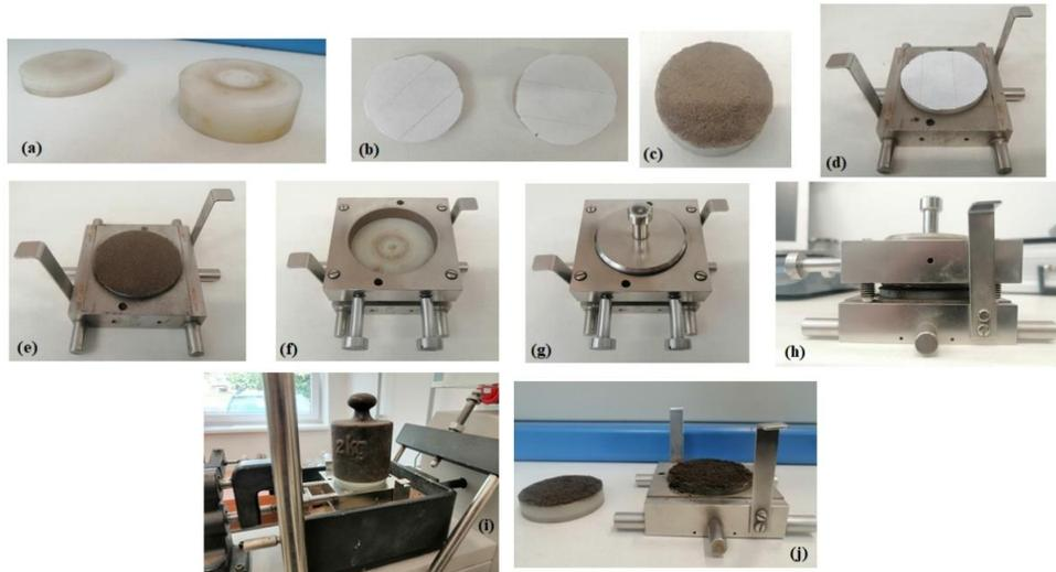
**Fig. 5.1.** (a, b) show the prepared teflon cylinders, with double face tape used on them, (c) shows the soil sticking on the other face of the tape, this sample is prepared for the upper frame, (d, e) lower frame teflon with soil prepared on it, (f, g, h) frame assembled, shearing zone seen in h, (i) Box installed in the shear machine with normal load applied - all masses applied are considered (with the teflon piece mass), (j) soil of high moisture content on the tape face.
