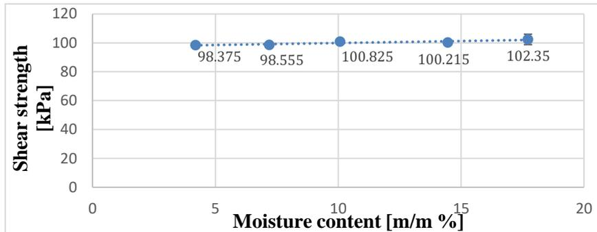
**Fig. 3.7.** Shear strength as function of moisture content (70 kg/223.68 kPa initially applied load/stress, and 30 kg/95.86 kPa is used with shearing).
