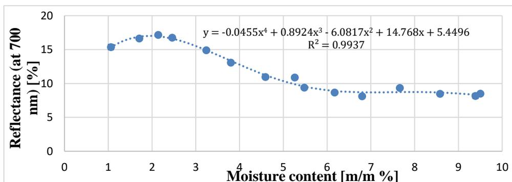
**Fig. 2.5.** Colour reflectance (at 700 nm) as function of moisture content, loam sand soil (90.50 % sand, 3.20 % silt, 6.30 % clay).
