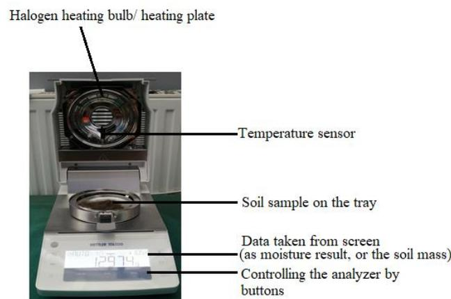
**Fig. 2.2.** Soil prepared on the moisture analyzer tray before closing the cover (HE 53 moisture analyzer).
