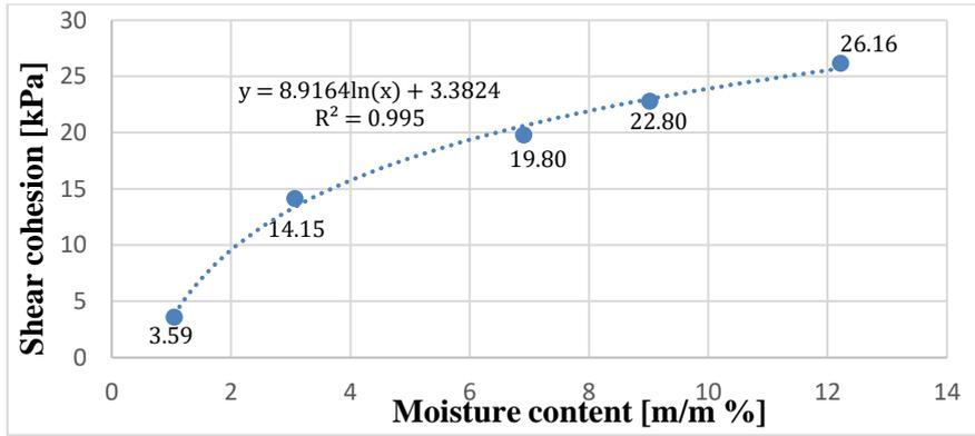
**Fig. 3.3.** Loam sand soil shear cohesion as function of moisture content.
