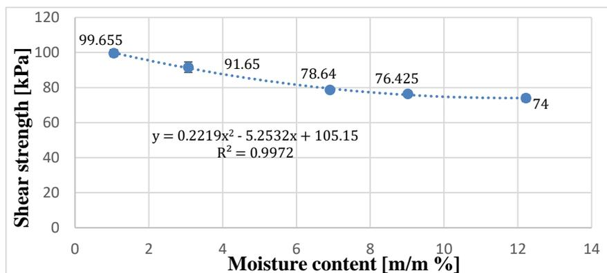
**Fig. 3.2.** Loam sand soil shear strength as function of moisture content (70 kg/223.68 kPa initially applied load/stress, and 30 kg/95.86 kPa is used with shearing).
