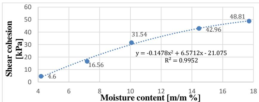
**Fig. 3.8.** Shear cohesion as function of moisture content.
