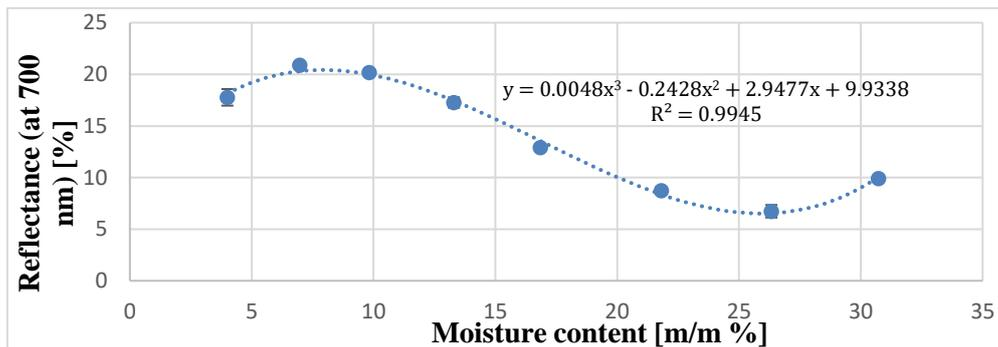
**Fig. 2.7.** Colour reflectance (at 700 nm) as function of moisture content, silty clay soil (3.34 % sand, 52.05 % silt, 44.61 % clay).
