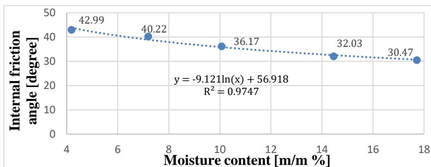
**Fig. 3.9.** Internal friction angle as function of moisture content.
