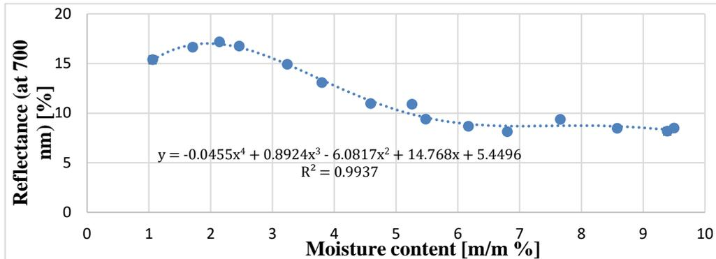
**Fig. 7.1.** Colour reflectance (at 700 nm) as function of moisture content, loam sand soil (90.50 % sand, 3.20 % silt, 6.30 % clay), the equation is of the curve in the range 1.06 to 6.80 %.
