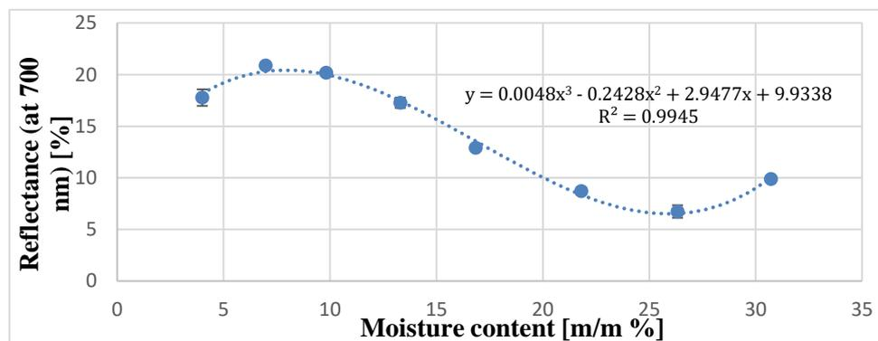
**Fig. 7.2.** Colour reflectance (at 700 nm) as function of moisture content, silty clay soil (3.34 % sand, 52.05 % silt, 44.61 % clay).
