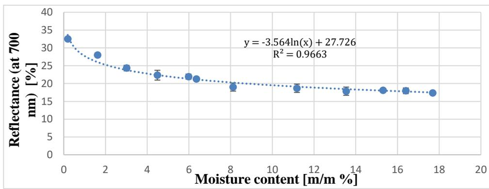
**Fig. 7.3.** Colour reflectance (at 700 nm) as function of moisture content, sand soil (94.53 % sand, 4.78 % silt, 0.69 % clay).
