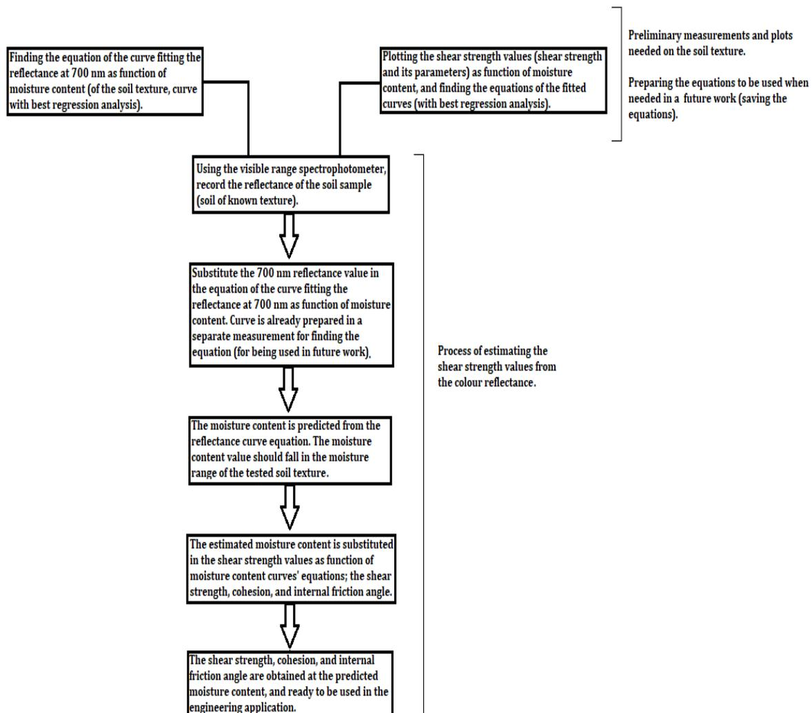
**Fig. 4.1.** Flowchart showing the process followed for predicting the shear strength values from the colour reflectance.
