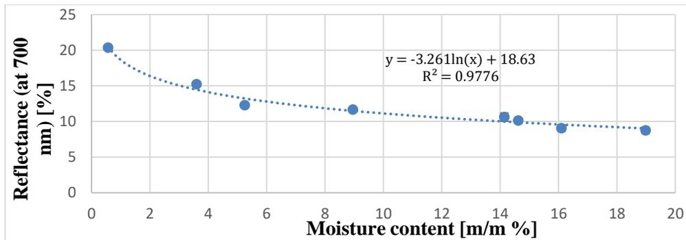
**Fig. 2.6.** Colour reflectance (at 700 nm) as function of moisture content, sand soil (95.68 % sand, 2.12 % silt, 2.21 % clay).
