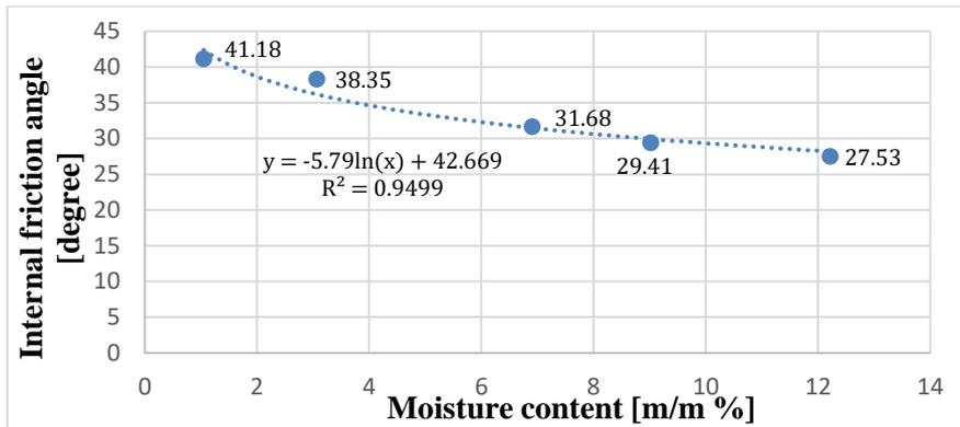
**Fig. 3.4.** Loam sand soil internal friction angle as function of moisture content.
