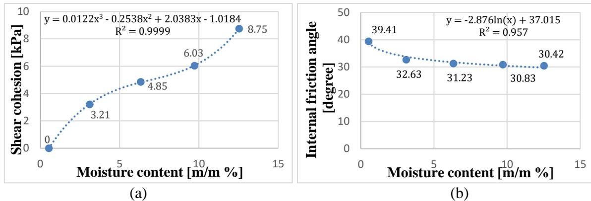
**Fig. 3.6.** (a) Sand soil shear cohesion as function of moisture content, (b) internal friction angle as function of moisture content.
