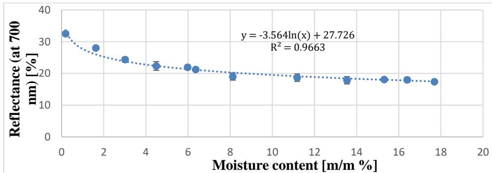
**Fig. 2.3.** Colour reflectance (at 700 nm) as function of moisture content, sand soil (94.53 % sand, 4.78 % silt, 0.69 % clay).
