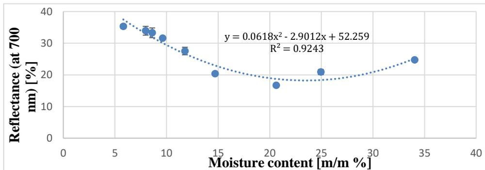
**Fig. 2.4.** Colour reflectance (at 700 nm) as function of moisture content, silty clay loam (14.07 % sand, 47.46 % silt, 38.47 % clay).
