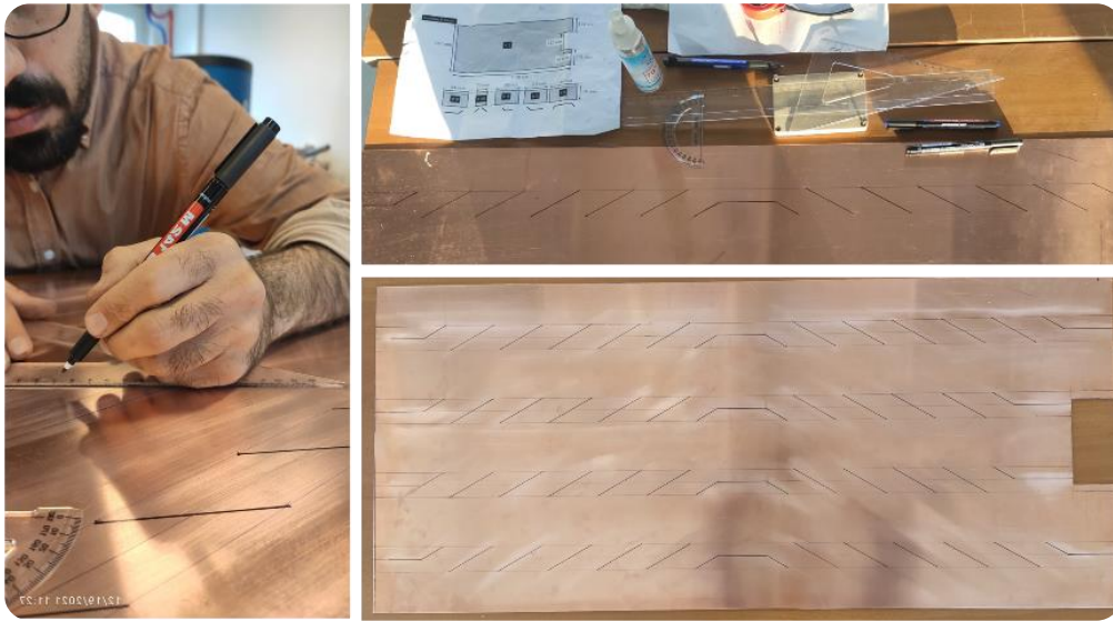
Fig. 3.13. Drawing of the exact positions of the fins
