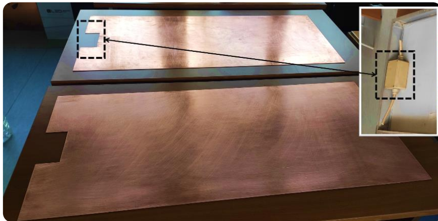
Fig. 3.9. Copper absorber of the research modules
