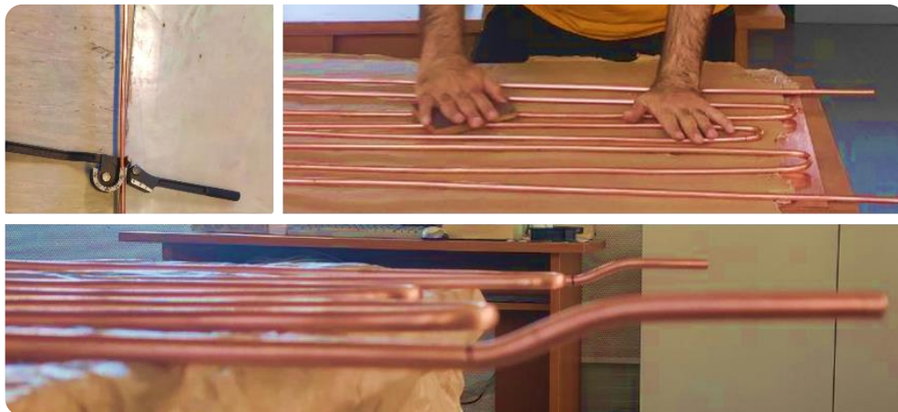
Fig. 3.14. Creation of the serpentine tube
