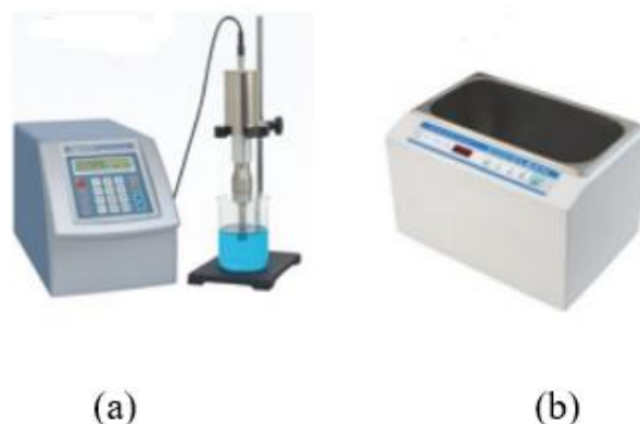
Fig 2.9. Ultrasonics types. (a) Probe (b) Bath
