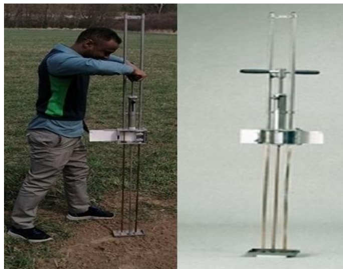
Figure 3.5. Cone penetrometer (06.02 Penetrograph) while the measurement.
