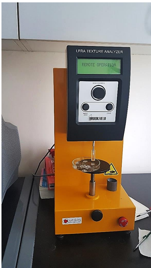
Appendix-Figure 2: Brookfield LFRA 4500 Texture Analyzer
