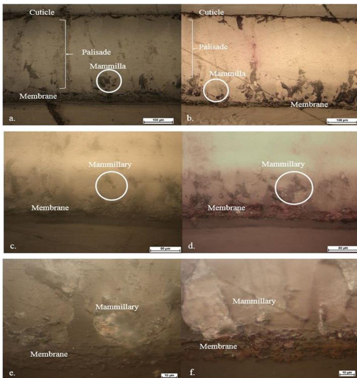
Figure 32. Polarization microscope images of thin sections from (a, c, e) the control eggshell and (b, d, f) eggshell with 2 g/L RBV-5R adsorbed.
