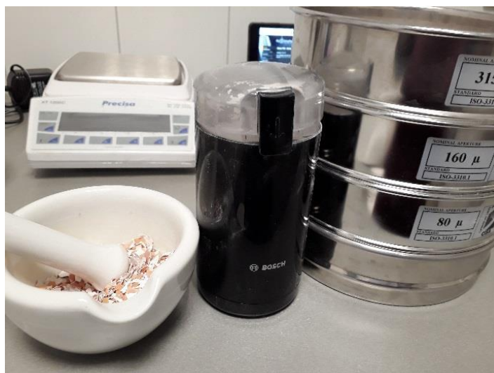
Figure 10. Preparation of eggshell powder.
