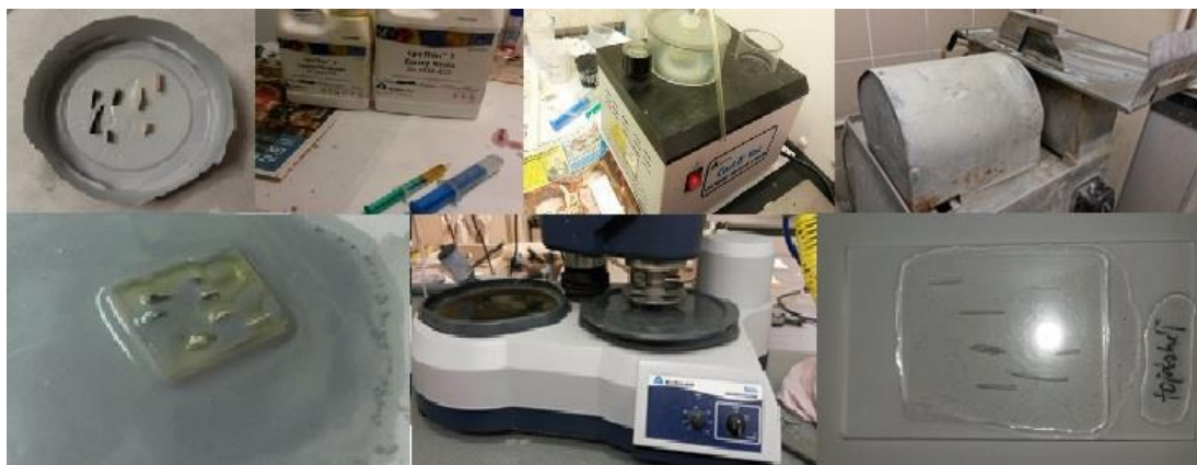
Figure 9. Preparation of eggshell thin section.
