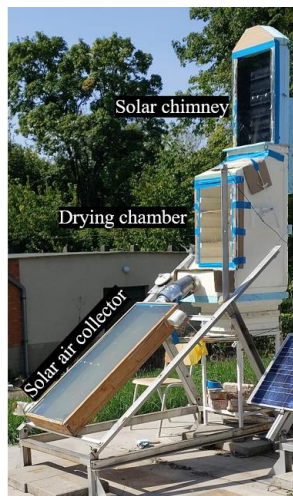
Fig. 1. Complete view of a novel indirect solar dryer
