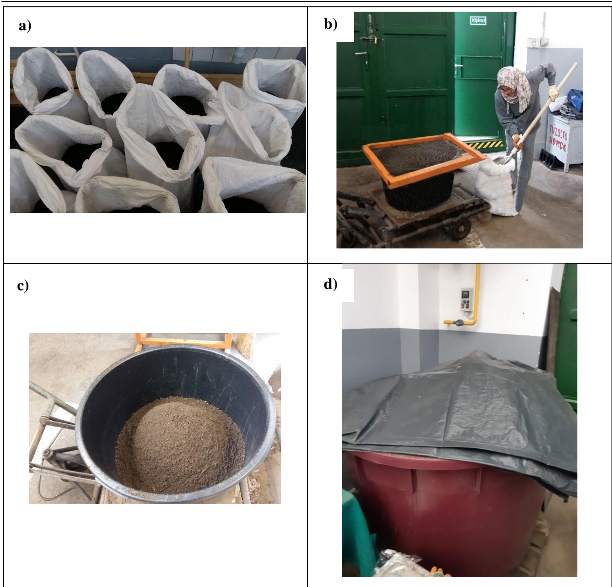
Fig. 3.5. Soil preparation: a) Soil brought from the field, b) Sieving the soil, c) Purified soil and d) Stored the soil
