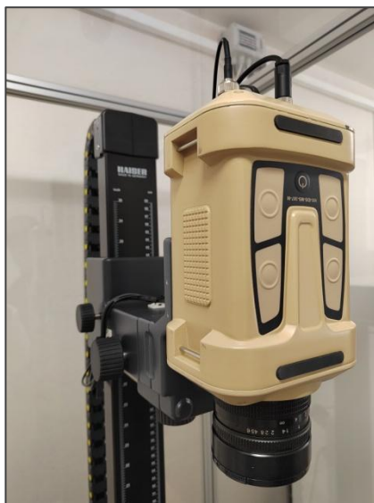
Figure 1: The custom-built thermal camera used since 2020
