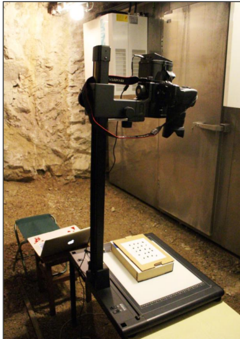
Figure 2: Thermal imaging of seeds placed on a cardboard in the mine passage of the Esztramos Mountain
