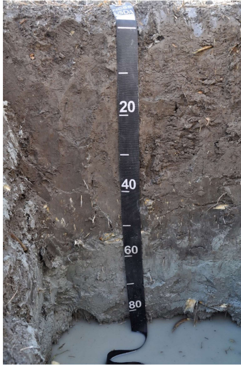
Figure 1. The soil profile at the eastern end of the sample area clearly shows the reductive conditions in the depth and the groundwater level within 1 meter of the surface.
